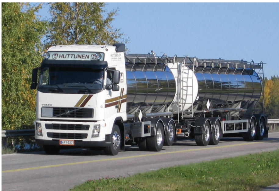
Figure 2: Truck and full trailer combination for chemical transports in Finland.
