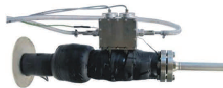
Figure 1: Microwave Transmissions and Reflection cell from hf-Sensor.
