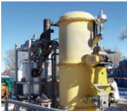
Figure 3: Transportable fluid-bed pyrolyser from Virginia Polytechnic Institute and State University.
