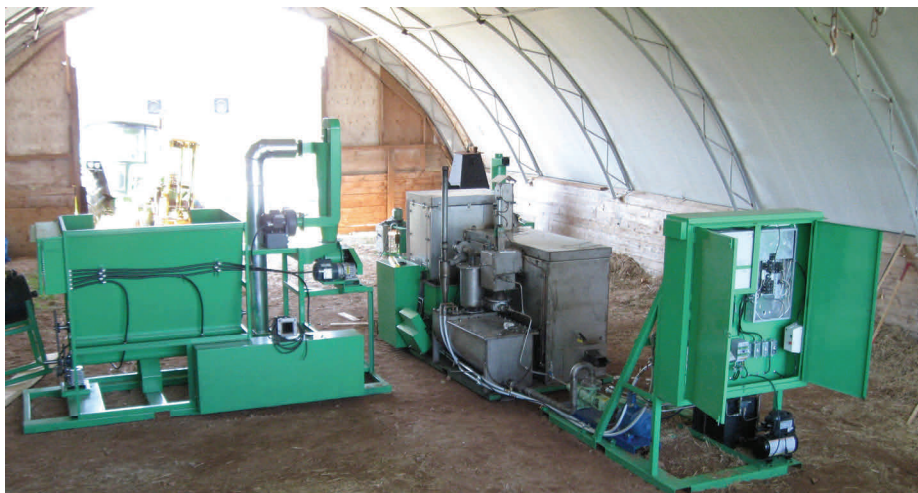
Figure 1: ABRI-Tech's 1t/d mobile pyrolysis system.
