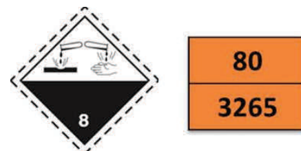
Figure 1: Pyrolysis oil labelling for transportation.
