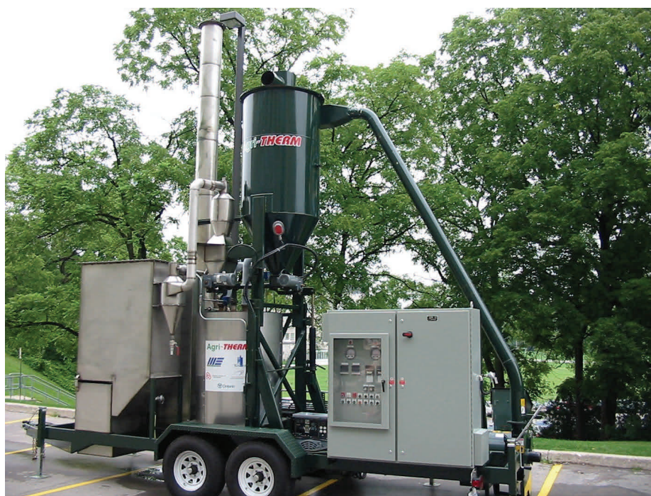
Figure 2: The Agri-Therm field deployable unit (up to 5t/d).
